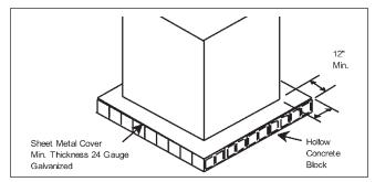
Figure 4. Typical Combustible Floor Installation.
